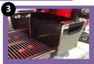
Pull the grounds drawer completely forward and out of the machine, empty all the used coffee from inside. At the end of the day wash and dry.
