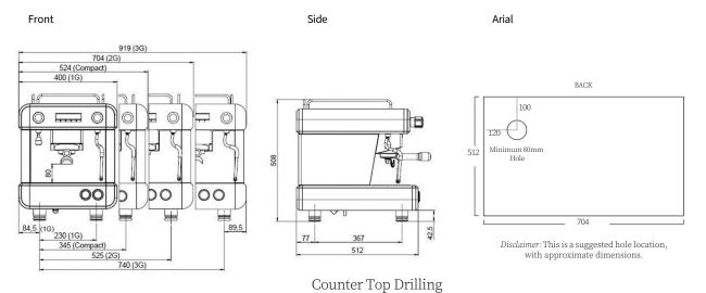
When preparing to drill your counter top, the key point to consider is that the waste hose needs a continuous drop. You will need a minimum of an 80mm hole, all of the utility cables and hoses are flexible therefore a central position provides best access and minimises drilling.
